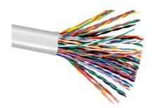
Category 3 UTP 100 MHz Cable Consists of HDPE Insulated 24AWG Solid Bare Electrolytic Grade Copper Conductors Twisted as 1 Pairs, PVC Outer Jacket. This Cable is Suitable for transmitting data, telephone and television signals at frequencies up to 100 MHz
