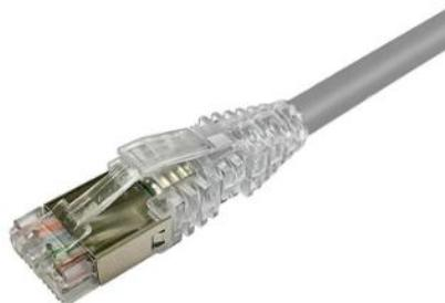
High Speed 10 Gigabit S/FTP Patch Cable Grey, LSZH, C6A delivers optimal transmission and networking performance with reduced insertion loss and Alien Crosstalk. They have high performance components available in broad range of lengths and designed to meet or exceed all Cat6A specifications. 26AWG conductors are securely mated with Shielded RJ45 plug design to deliver superior performance.
