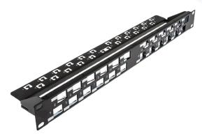
The rack mountable Angled Staggered Patch Panel offers fast and reliable installation of Unshielded cables. A rear cable management bar is supplied which acts as stress reliever for terminated cables. Angled position provided to Keystone outlets to reduce strain relief on connected patch cords. Patch panel is provided with mini cable ties, cage nuts & rare cable management. The Jack to be ordered separately.
