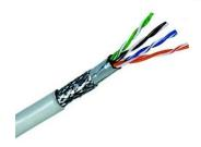
High Speed Gigabit Ethernet UTP 250 MHz Class E / Category 6 Cable Consists of HDPE Insulated 8 x 23AWG Solid Bare Electrolytic Grade Copper Conductors Twisted as 4 Pairs, Al-Mylar Tape with Drain Wire, overall Aluminum braiding and FRPVC Outer Jacket. This Cable is Suitable for Gigabit Ethernet (1000Base-T) applications for High-Speed Data, Voice & Video Signals over LANs, Server Farms and Other Bandwidth Sensitive Indoor Applications.
