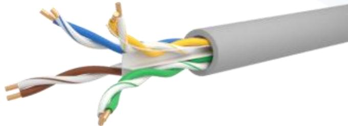
High Speed Gigabit Ethernet UTP 250 MHz Class E / Category 6 Cable Consists of HDPE Insulated 8 x 23AWG Solid Bare Electrolytic Grade Copper Conductors Twisted as 4 Pairs, Rip Cord and LSZH Outer Jacket. This Cable is Suitable for Gigabit Ethernet (1000Base-T) applications for High-Speed Data, Voice & Video Signals over LANs, Server Farms and Other Bandwidth Sensitive Indoor Applications.
