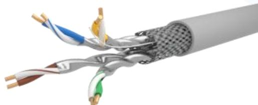
High Speed 10Gigabit Ethernet S/FTP 500 MHz Class EA / Category 6A LSZH Cable is produced using 8x23 AWG Solid Bare Copper Conductors. Every pair is separately shielded – pairs in metal foil (PIMF). The twisted pairs are covered with a braided screen (S/FTP) which guarantees outstanding shielding properties and then LSZH Outer Sheath. It supports 10/100/1000Base-T, 155Mbps ATM, IEEE 802.3an (10GBase-T) Standard.
