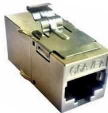
Shielded Inline Coupler, C6A avoids the need for rear termination and allows two patch cables to be connected directly, with no tools required. This inline coupler fits in any keystone wall plate, Patch panel, or surface mount box. Rated for Cat6A network, allows for bandwidth up to 10Gigabit per second.
