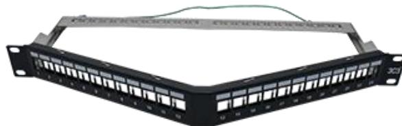
Patch Panel V-shaped Angled, 1U offers fast and reliable installation of shielded cables, a rear cable management bar is supplied which acts as stress reliever of terminated cables. Each port of the panel is numbered and has designated label area for clear port identification.
