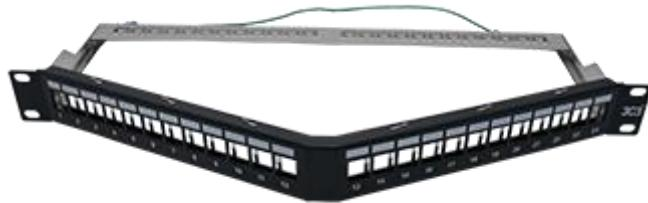
Patch Panel V-shaped Angled, 1U offers fast and reliable installation of shielded/unshielded cables, a rear cable management bar is supplied which acts as stress reliever of terminated cables. Each port of the panel is numbered and has designated label area for clear port identification.
