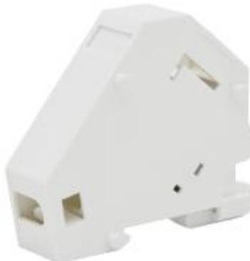
Din Rail Mountable Module for shielded Keystone jack to be mounted on the standard Din rail. The grounding contacts the outer casing of the keystone jack to give a secure earthing point through to the Din Rail
