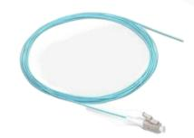
Fiber Optic pigtail is used in permanent connection between patch panels and incoming cables. Pigtails are pre-constructed with connectors. Connector options include LC, SC, FC, ST, MTRJ, and E2000. These are based on 900micron tight buffered cores and suitable for internal use only.
