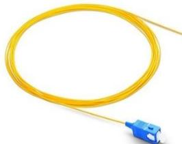
Fiber Optic pigtail is used in permanent connection between patch panels and incoming cables. Pigtails are pre-constructed with connectors. Connector options include LC, SC, FC, ST, MTRJ, and E2000. These are based on 900micron tight buffered cores and suitable for internal use only.
