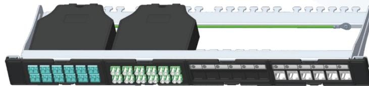
The High-Density Hybrid panel accepts either or both copper and fiber modules. The Panels are designed with 4 cutouts, offer fast and reliable installation, reduces required rack space and provides future proofing in system design; a rear cable management bar is supplied which acts as stress reliever for terminated cables. Patch Panel includes mini cable ties, cage nuts and rare cable management.
