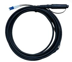
The Rugged Fiber Optic Patch cords are basically Fiber Optic Patch Cords suggested for more rugged harsh environments. The spiral steel tape provides additional crush resistance and rodent attack prevention. The patch cord can be deployed in Remote Radio Head cell tower applications and connection between distribution box and RRH.
