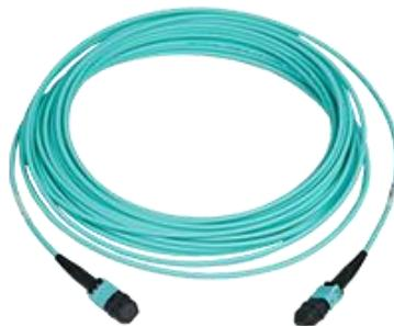
MPO Fiber Cabling System is ideally suited for a high-density environment that demands space saving and innovative cable management solutions. The MPO connector offers up to 12 times the density of standard connectors providing significant space and cost savings. MPO Patch Cord utilizes precision molded MT ferrule, with metal guide pins and precise housing dimensions to ensure fiber alignment when mating.
