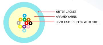
Indoor fiber optic cables are tight buffer design, usually it consists of aramid yarns distributed over-which is used to strength the cable structure and to resist high tension, FR-LSZH outer jacket makes perfect for indoor applications.
