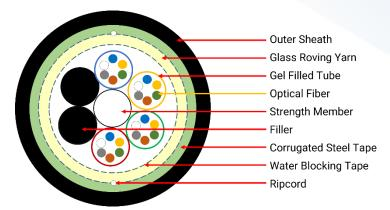
The Outdoor fiber optic cables are PBT Multi loose tube with colored fiber cores. The constructions are of water-blocking gel material with Non-Metallic Central Strength member & ECCS armoring. This cable has HDPE outer jacket which makes it perfect for outdoor applications.
