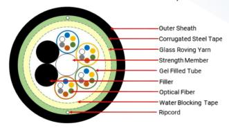
The Outdoor fiber optic cables are PBT Multi loose tube with colored fiber cores. The constructions are of water-blocking gel material with Non-Metallic Central Strength member & ECCS armoring. This cable has LSZH outer jacket and makes it perfect for outdoor applications
