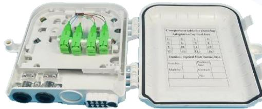
Wall Mount Planar Light Wave Circuit (PLC) Splitters comes in PC + ABS Material enclosure with block less splitter assembly. It supports a variety of spectra 1:2, 1:4, 1:8, 2:2, 2:4, 2:8. PLC Splitter is type of optical power management device that is fabricated using silica optical waveguide technology. It is small size, high reliability, wide operating wavelength range and good channel uniformity.
