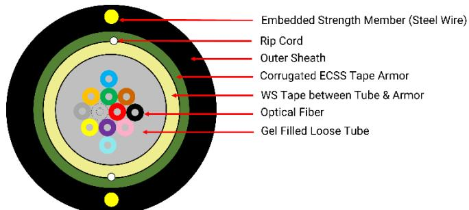
Single Mode Uniloose tube, single sheath ECCS tape armored optical fiber cable is suitable for duct and aerial applications. Fiber cable is perfectly suited for both gigabit Ethernet and 10 gigabit Ethernet campus and backbone applications.
